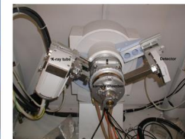
XRD diffractometer Philips X`Pert Pro with high temperature chamber up to 1600 °C
