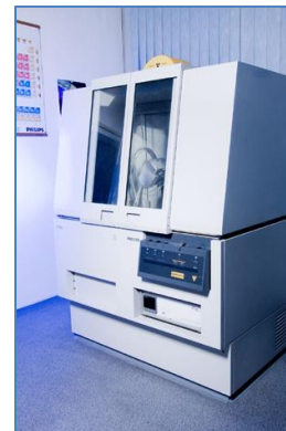
XRD diffractometer Philips X`Pert Pro with high temperature chamber up to 1600 °C
